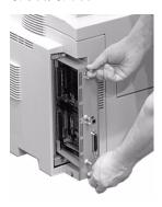
2. Reinstall the thumbscrews at the top and bottom of the board.
